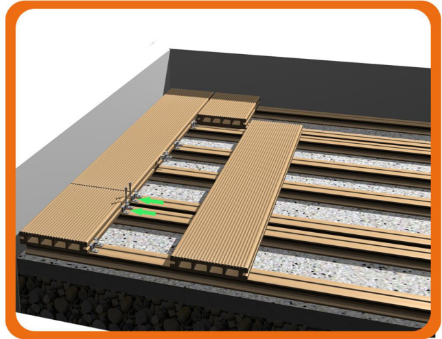
III 、 The end of each decking profile needs to be put on each keel/joist.
