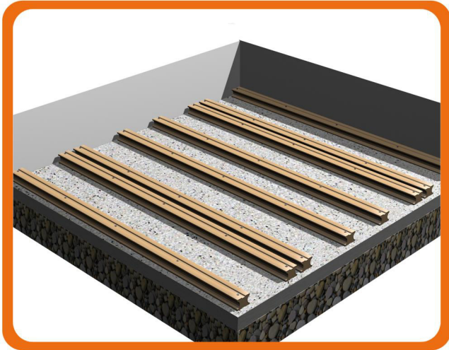
I 、 The decking conjunction place needs two pcs keels/joists
